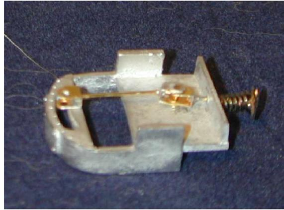
3. Drill the buffer casting with a hole of about 0.8 - 1mm dia, in the centre of the inner upright panel, and fit the coupling. You could add a short spring (a short length of old ballpoint pen spring) and with a washer, or offcut of brass secure it behind the buffer casting. As before do not rely on solder alone, but bend the pin so as to form a mechanical anchorage.
