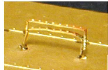
15. Now fold up the ends, and then the sides so that the corner plates overlap the ends. Working round from corner to corner solder the tops with a small dab of solder (making sure that the two parts are level with one another as the floor can distort). Then run some flux up the inner corner and follow with a tinned iron. Do not use a large dollop of solder, or try to form a fillet. This will only bleed out and spread over the details on the outer face of the model.
