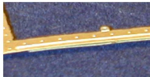
10. Turn the component back and fold the strap around the staple to form a hinge. Note that there is a rivet head on the strap. Flux the end of the strap away from the hinge hold down it down with the tip of a screwdriver, file or whatever comes to hand and touch the tinned iron to the end of the strap and the door beneath. The solder should flash between the two and stop where they part to form the hinge.
