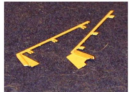
17. These and the other ribs are fitted by means of the double tabs through the sides. The tabs are bent to either side on the inside of the van. It is easiest to do 3 or 4 at a time, including those on the ends (**Parts 16**) and the side (**Parts 17**) and then securing them with a dab of flux and a touch of solder. Again beware of allowing the solder to bleed through to the front.
