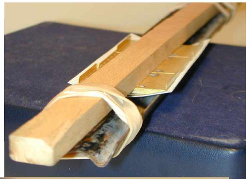
27. The corrugated iron is held on with straps (**Parts 26**) and 5 bolts each. The central one has an eye for the emergency brake cord. After positioning the strap, drill right through the roof at one end. Set a pin in position and solder it from beneath. Then fix the other end, and finally the three central holes. However the middle pin can be made up from an offcut pin, bend it round a suitable former or round nosed pliers, and solder the inside end of it too.
