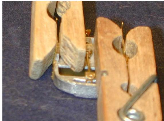
5. The chassis (**part 4**) is folded up, or down as shown. At this stage it is better not to fold the brakes down as they are too vulnerable,
